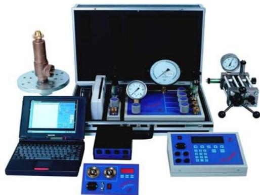
It was used for conventional testing of safety valves as well as pressure and temperature sensor calibration.
