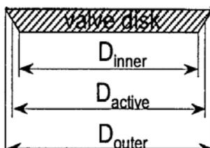
The most common approach is to presume that the active valve disc diameter (which is the basis for the value  $A_{seat}$ ) is equal to the average of the inner and the outer valve disc diameter.
