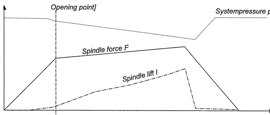
As indicated in the introduction the curves have a **characteristic point** where their **gradient abruptly changes at the same time** - at the **moment when the valve starts popping up** (see the schematic diagram enclosed).
