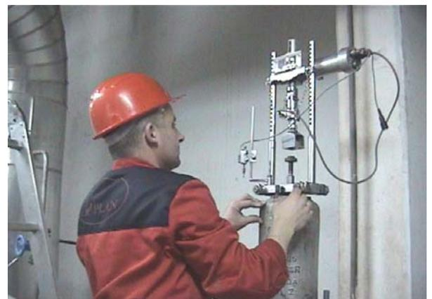
The operation of LEGATEST is controlled from PC which must be connected to the motor housing by a single cable.
