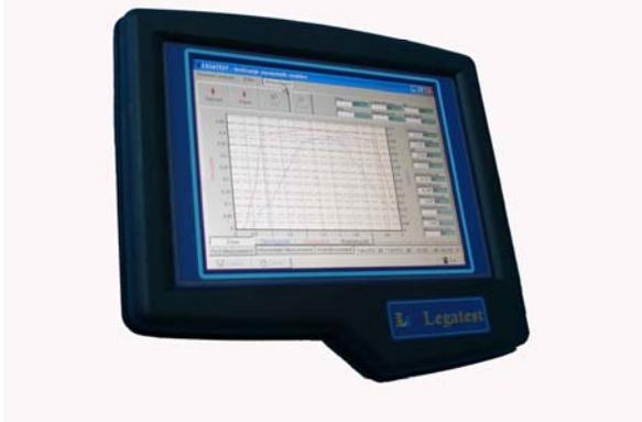
By pressing button START testing sequence will be started and construction motor begins to move. When construction starts to strain, increase of force and lift can be observed. When valve opens, the pressure in the system starts to fall. On right side of display we can observe the numeric values of all parameters in every instant of time.
